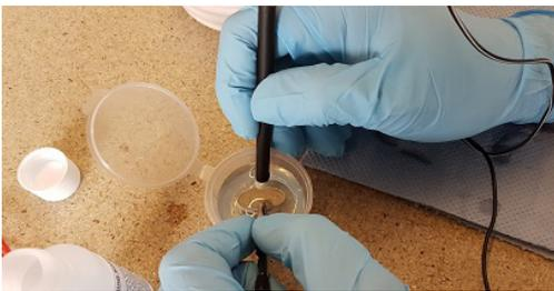
Continue plating to get a good coverage. Dip the item in the hot water from time to time to keep the temperature up. You can speed up the plating by using the cup to tank plate. While “tank” plating you will see bubbles rising from the brush and the item being plated.
