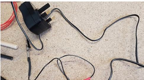
The power supply has a voltage adjustment. Set it to between 4.5 and 7.5 volts. Attach a plating brush or detail pen to the red terminal. Connect a crocodile clip to the black terminal.
