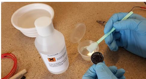
Now activate the surface of the item with the acid pickle. Rub the item using the swab and acid pickle. Do this for a couple of minutes, then rinse the item.
