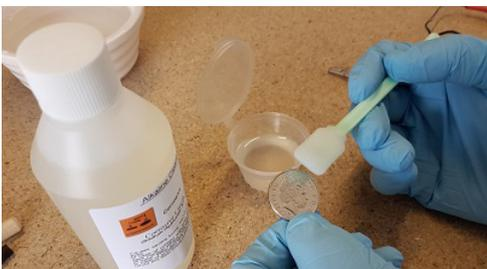
With our gloves on we first have to degrease the item. Use the swab and the alkaline degreaser to clean the item. To test that the grease is gone, hold the item under a trickle of water. If the water beads there is grease present on the surface. Carry on cleaning.
