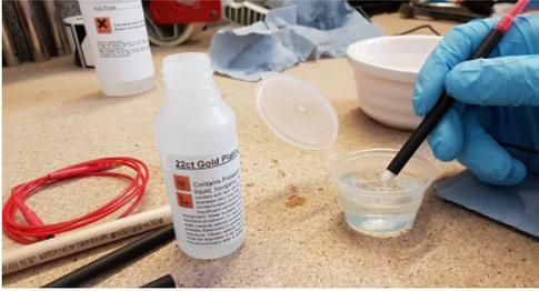
Now we can start plating. Take a small mug and fill it with hot water which we will use to raise the temperature. Pour some gold electrolyte into the small plastic cup.
